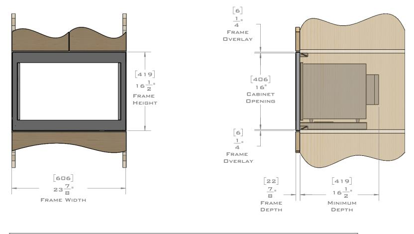
EUROTRIM MICROWAVE TRIM KITS ARE SUPPLIED COMPLETE WITH ALL HARDWARE REQUIRED. OUR UNIQUE STOPADS ALLOW FOR A PERFECT INSTALLATION EVERY TIME. -FOR VENTILATION A 6 SQUARE INCH (39 SQ.CM.) CUT OUT MUST BE PLACED IN THE REAR OF THE CABINET. FAILURE TO DO SO MAY CAUSE DAMAGE TO THE MICROWAVE OVEN AND OR CABINET. DIMENSIONS IN [ ] ARE MILLIMETER
