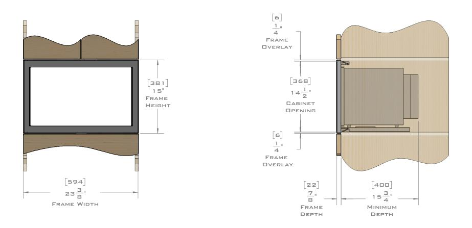
EuroTrim microwave trim kits are supplied complete with all hardware required. Our unique STOPADS allow for a perfect installation every time. -For ventilation a 6 square inch (39 sq.cm.) cut out must be placed in the rear of the cabinet. Failure to do so may cause damage to the microwave oven and or cabinet.
