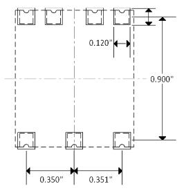
For best signal integrity, do not run traces beneath the part, and ensure the area under the board is ground plane.
