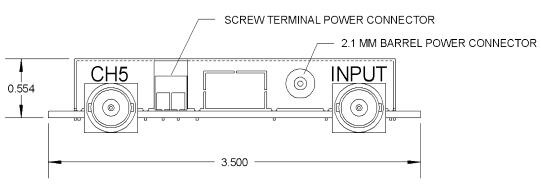
All dimensions are in inches with a tolerance of ±0.020°
