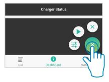
Access the Charger Optipons menu by tapping on the left bottom corner button of the Dashboard view
