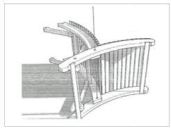
**1.** Lay the centre bench and back section on their side. Ensure the angle adjustment piece is seated on the bar.
