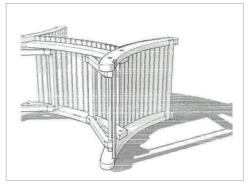
**2.** Repeat the process for the other end. Flip the piece over and repeat the process for the other side.
