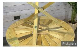
**3.** When all three legs are attached, open them up so the notched ends can reach and slot into place snuggly on the edges of the table support planks. Note: They do not go exactly in the middle of the support planks that they reach (see picture 3).
