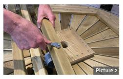
**2.** Finger-tighten the bolts to the legs and circular triple hinge, it is important to ensure that the angled cuts at the bottom of each leg face in the circular direction (see picture 2).
