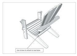
**3.** Attach the arms to the seat back and legs using 12 x torx screws.
