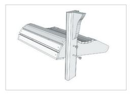
**1.** Attach the legs to the seat assembly using dome head bolts and affix using a washer
