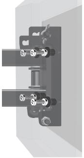
STEP 3 Install bracket with television to portable mounting plate: Attach as shown below.
