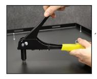
Install the tray by inserting the supplied rivets into the holes of the new, larger tray to the trail kitchen.
