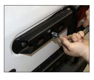
Fasten the hinge to the tailgate with the supplied M8 bolts.
