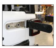
Remove the torx bolts connecting the stock tailgate hinge to the tailgate.
