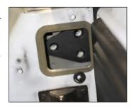
Remove the bolts connecting the stock hinge to the tub of the Jeep through the interior access panel.
