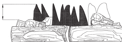
Figure 52– Correct Flame Pattern with Control Knob Set to High Flame
