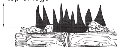
Figure 53– Incorrect Flame Pattern with Control Knob Set to High Flame
