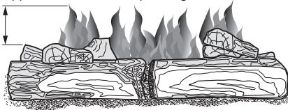
Figure 21 - Correct Burner Flame Pattern
