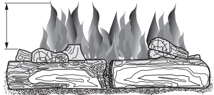
Figure 22 - Incorrect Burner Flame Pattern
