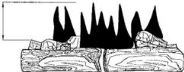
Figure 32 -Incorrect Flame Pattern with Control Knob Set to High (5)
