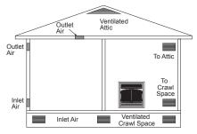
Figure 3 - Ventilation Air from Outdoors
