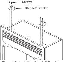
Figure 10 - Installing Standoff Brackets
