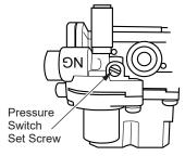
Figure 34 - Gas Regulator Pressure Switch
