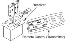
Figure 21 - Installing Batteries in Remote Control and Receiver
