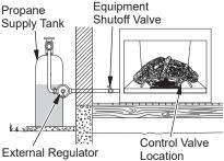
Figure 14 - Checking Gas Joints for Propane Gas
