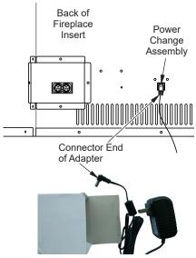
Figure 4 - Connecting to Power Supply
