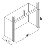
Figure 8 - Rough Opening for Wall Installation
