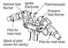
Figure 33 - Pilot Inlet Air Hole
