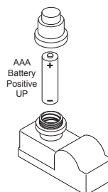
Figure 20 - Installing Battery in Ignitor
