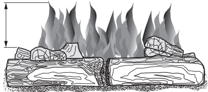
Figure 30 - Incorrect Burner Flame Pattern (Actual logs will vary from illustration.)
