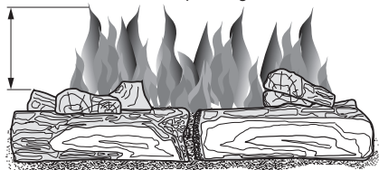
Figure 24 - Incorrect Burner Flame Pattern
