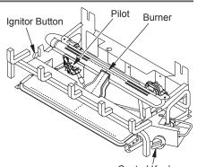
Control Knob Figure 1 - Vent-Free Log Chassis
