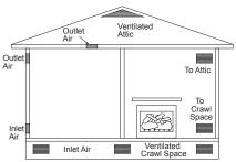
Figure 3 - Ventilation Air from Outdoors
