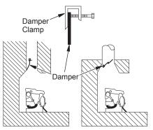
Figure 10 - Attaching Damper to Fireplace
