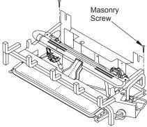
Figure 12 - Attaching Heater Base to Fireplace Floor
