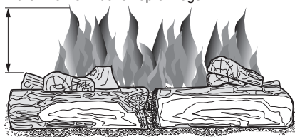
Figure 24 - Incorrect Burner Flame Pattern
