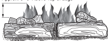
Figure 25 - Correct Burner Flame Pattern
