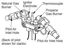
Figure 34 - Pilot Inlet Air Hole
