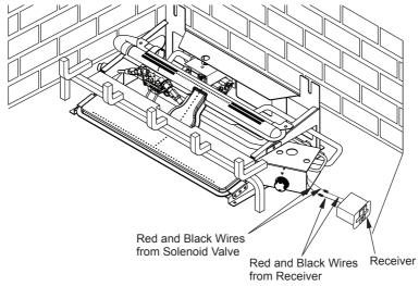
Figure 20 - Attaching Remote Receiver to Solenoid Valve
