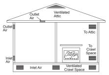
Figure 3 - Ventilation Air from Outdoors
