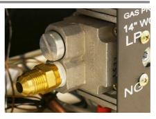
Use only the metal cap. DO NOT use an off the shelf 3/8" NPT pipe plug. This will damage the plungers located inside the regulator.
