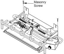
Figure 10 - Attaching Heater Base to Fireplace Floor
