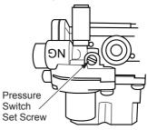
Figure 35 - Gas Regulator Pressure Switch
