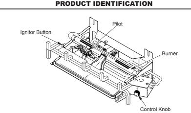
Figure 1 - Vent-Free Log Chassis
