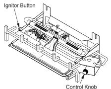
Figure 22 - Ignitor Button and Control Knob Locations
