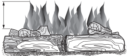
Figure 29 - Incorrect Burner Flame Pattern
