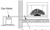
Equipment Shutoff Valve Figure 7 - Checking Gas Joints
