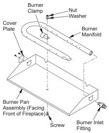
Figure 3 - Installing Burner
