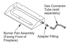
Figure 4 - Connecting Gas to Appliance
