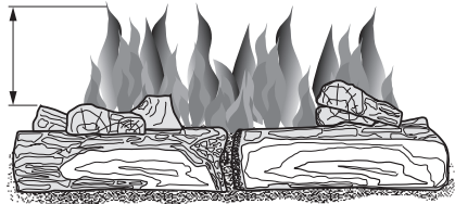
Figure 30 - Incorrect Burner Flame Pattern
