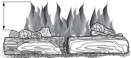
Figure 28 - Incorrect Burner Flame Pattern
