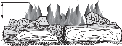
Figure 28 - Correct Burner Flame Pattern
