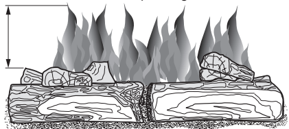
Figure 22 - Incorrect Burner Flame Pattern
