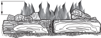
Figure 26 - Correct Burner Flame Pattern with Control Knob Set to HI (5)
