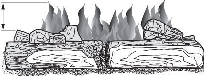
Figure 37 - Correct Burner Flame Pattern
