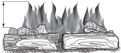
Figure 38 - Incorrect Burner Flame Pattern
