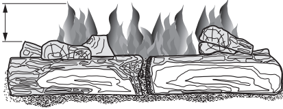
Figure 30 - Correct Burner Flame Pattern
