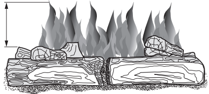
Figure 31 - Incorrect Burner Flame Pattern
