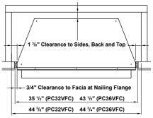
Note: Height of fireplace opening at facia to be 32 ½" (PC32VFC) and 36 ¾" (PC36VFC).
