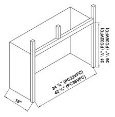
Figure 4 - Rough Opening for Installing in a Wall
