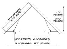
Figure 5 - Rough Opening for Installing in a Corner
