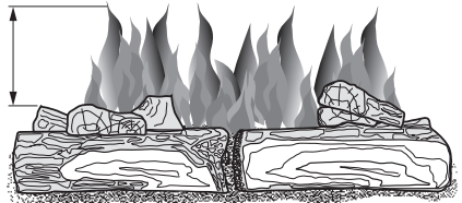
Figure 36 - Incorrect Burner Flame Pattern
