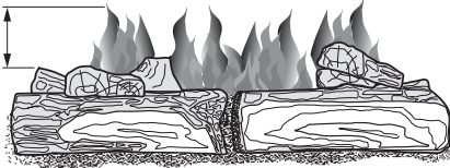
Figure 35 - Correct Burner Flame Pattern
