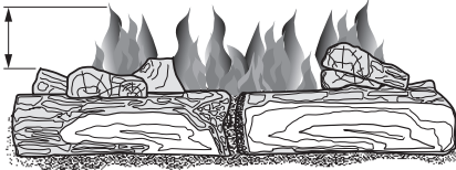
Figure 33- Correct Burner Flame Pattern
