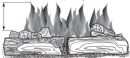
Figure 34 - Incorrect Burner Flame Pattern
