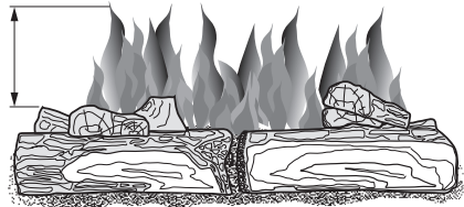
Figure 33- Incorrect Burner Flame Pattern with Control Knob Set to HI (5)
