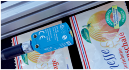
Thanks to two LEDs and powerful foreground suppression, the WTV4F, like V-optics, is able to reliably detect very flat objects.
