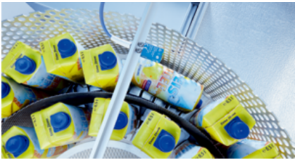
Thanks to the two different switching points, the WTB4F MultiSwitch can distinguish between standing and lying objects.
