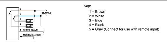
**Note:** Banner recommends that the shield wire (quick-disconnect cordsets only) be connected to earth ground or dc common. Shielded cordsets are recommended for all quick-disconnect models.
