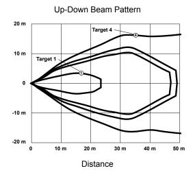
Weak Object (Radar cross section = 0.25 m<sup>2</sup>)
