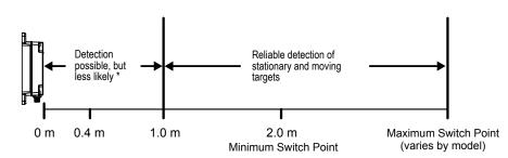
\*The specific detection range depends on the radar cross section and returned signal strength of the specific target. Moving targets provide a stronger signal and are more likely to be detected at closer distances. Typical stationary targets can be detected as close as 1 meter (3.3 feet). Typical moving targets can be detected as close as 0.4 meters (1.3 feet).
