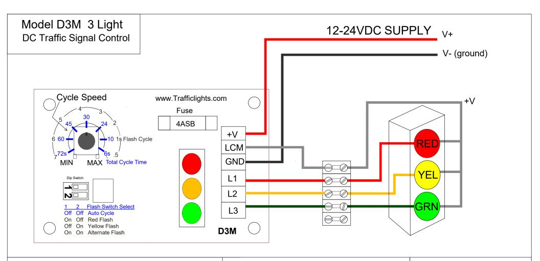
D3 - 3 Light DC Traffic Signal Sequencer, D3E-3 Light DC RR Block Signal Sequencer, Adjustable speed cycle with adjustable flash modes. Speed control is read once per cycle prior to Red light phase. F or DC Loads, LED or Incandescent 0 to 4A per channel.
