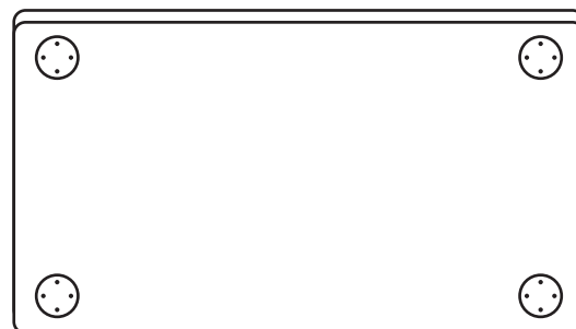
RECOMMENDED FLANGE PLACEMENT
