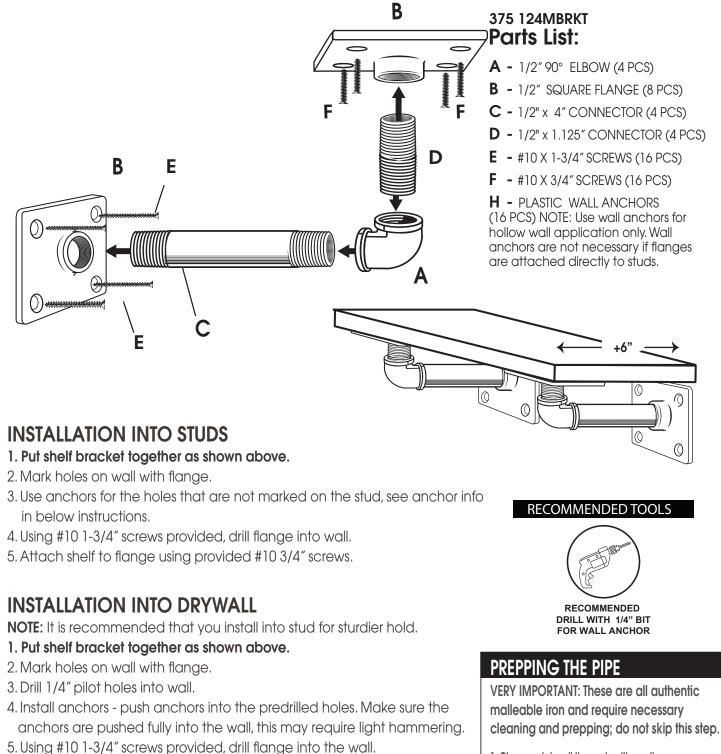
6. Attach shelf to flange using provided # 10 3/4" screws.
