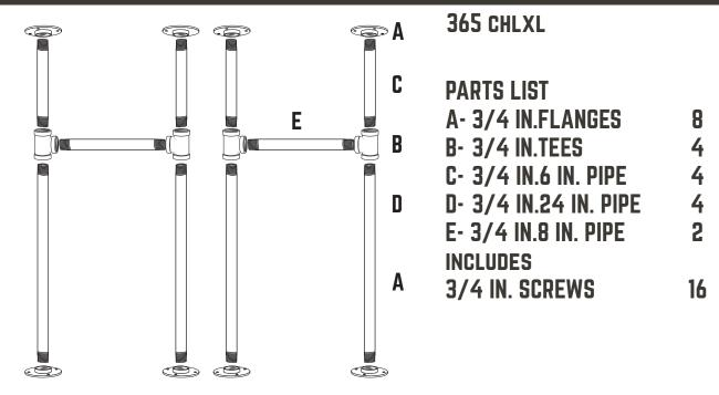
This kit is made of industrial grade authentic pipe. It is coated in oil post production to prevent rust. The kit should be cleaned and sealed to prevent rusting. See Clean and Seal sheet for more information on cleaning and sealing your pipe kit or watch the clean and seal video on the listing.
