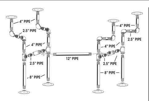
This kit is made of industrial grade authentic pipe. It is coated in oil post production to prevent rust. The kit should be cleaned and sealed to prevent rusting. See Clean and Seal sheet for more information on cleaning and sealing your pipe kit.
