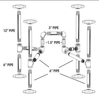
This kit is made of industrial grade authentic pipe. It is coated in oil post production to prevent rust. The kit should be cleaned and sealed to prevent rusting. See Clean and Seal sheet for more information on cleaning and sealing your pipe kit.
