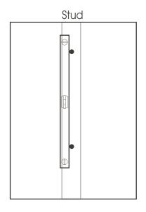
6. Using a 2' or 4' level, mark the top hole for the other bracket assembly in the center of the stud where it will be installed. This mark needs to be level with the first top hole mark. Mark the bottom hole the same way; level with the first bottom hole mark.
