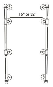
5. Place a barcket assembly against the wall in the desired location, with the top hole of the flange set in the center of the stud. Mark the hole with a pencil. Now mark the bottom hole of the bottom flange. Place a level between the top mark and the bottom mark. Adjust position of the bottom mark so it is vertically level with the top hole mark.
