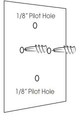
9. Install fully assembled bracket assemblies onto the wall with provided screws.
