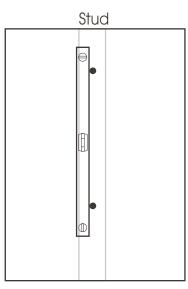
6. Using a 2' or 4' level, mark the top hole for the other bracket assembly in the center of the stud where it will be installed. This mark needs to be level with the first top hole mark. Mark the bottom hole the same way; level with the first bottom hole mark.
