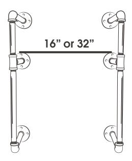
5. Place a barcket assembly against the wall in the desired location, with the top hole of the flange set in the center of the stud. Mark the hole with a pencil. Now mark the bottom hole of the bottom flange. Place a level between the top mark and the bottom mark. Adjust position of the bottom mark so it is vertically level with the top hole mark.
