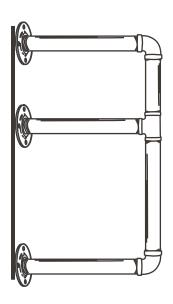
4. It is strongly recommended that the brackets are fastened to wall studs or a wood/metal backing plate. Studs are 1 1/2" wide and are generally located 16" apart, so the bracket assemblies need to be either 16" or 32" apart. Locate and mark the center of the studs with a stud finder (not included).
