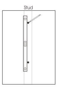
6. Using a level, mark the top hole for the other bracket assembly in the center of the stud where it will be installed. This mark needs to be level with the first top hole mark. Mark the bottom hole the same way; level with the first bottom hole mark.
