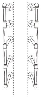
3. Make sure all flange faces are touching the flat surface evenly, this will assure that there are no gaps between any of the flanges on the wall. If flanges are not touching flat surface evenly, adjust accordingly by tightening or loosening flanges.
