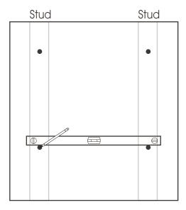
7. Hold the bracket assembly against the wall with the top and bottom mark lined up in the flange holes. Mark the remaining flange holes with a pencil. (NOTE: It is mandatory to use all 12:00 and 6:00 positioned flange holes to attach bracket to studs).
