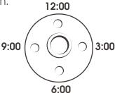
2. Set the assembled brackets side by side with the face of the flanges on a smooth, flat surface. See figure to the right. Make sure all flanges line up evenly side by side, this will help to assure your shelves on both sides are even. If flanges do not line up, adjust pipe accordingly by tightening or loosening.
