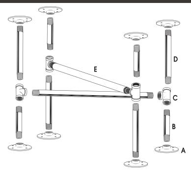
This kit is made of industrial grade authentic pipe. It is coated in oil post production to prevent rust. The kit should be cleaned and sealed to prevent rusting. See Clean and Seal sheet for more information on cleaning and sealing your pipe kit.
