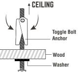
Tighten machine screws in order to bring board flush to the ceiling.
