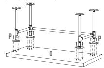
**STEP 3** Attach another wood piece using wood screws.
