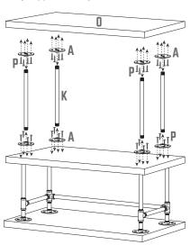
STEP 5 Assemble flanges, side-out elbows, 90° elbows, nipples, and flanges together, then attach to the assembled parts using wood screws.
