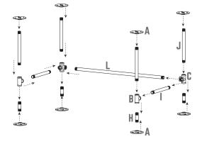
STEP 2 Attach the assembled parts to the wood piece, then align and attach 4 flanges to the bottom of wood piece using wood screws.
