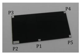
Figure 1 Airgain N703LTSTM embedded surface-mount LTE antenna P1: Feed-pin. P2: GND-pin, P3-P5: Soldering pins
