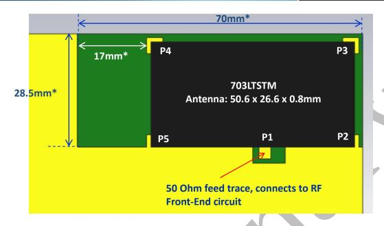
Figure 5 Airgain N703LTSTM LTE antenna mounted on PCB
