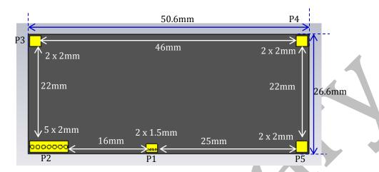
Figure 4 Airgain N703LTSTM antenna footprint and dimensions
