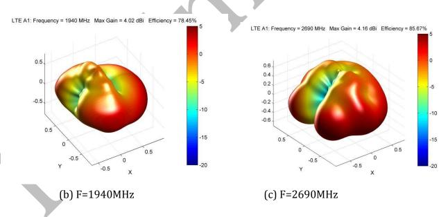
Figure 3 Airgain N703LTSTM antenna radiation patterns
